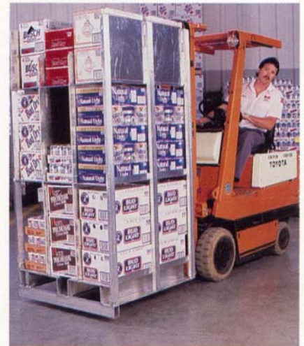
3. The fully loaded MultiPak Rack is moved by forklift to awaiting vehicle.
